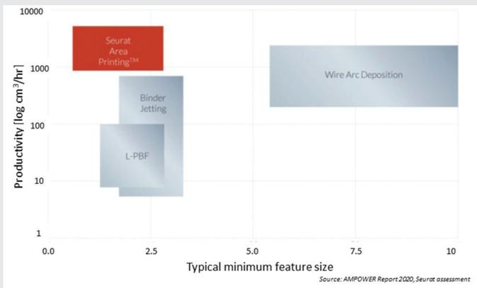
Figure 2- A comparison of productivity and feature size for different LAM techniques stainless steel).
